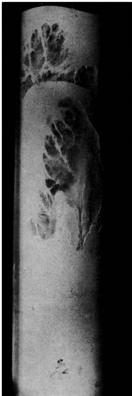
Fig. 8. Collapsing gas pockets. 3.75-in. column, inclined 10 deg., run 13, 200-mesh alumina.
