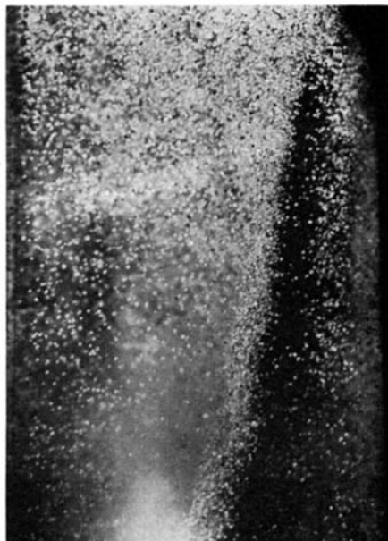
Fig. 1. Free-bed fluidization of 0.028-in. beads; run 5. Height of view = 5.5 in.
